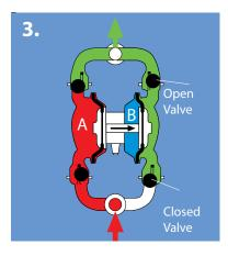
The process continues by again creating pressure in region B, this time expelling product from the pump while drawing in new product into chamber A where simultaneously a low pressure has been generated.
