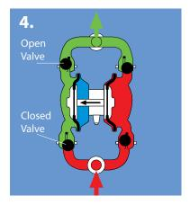
The cycle repeats by alternately producing pressure in regions B and C while the pump is in operation.
