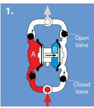
On start-up, pressurized air in region B (acting via connected diaphragms) lowers the pressure in chamber A.
