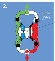
positions of inner pistons switch the control valve between alternating phases.
